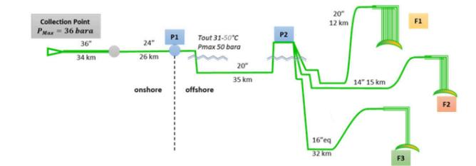
Fig 4. Injection Network Schematic with key nodes (P1, P2)
