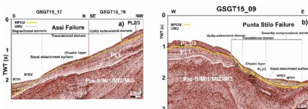
Fig. 3. High-resolution 2D seismics (from RITMARE) showing seismo-stratigraphic units affected by slope failures, the so-called AF (a) and PSF (b).
