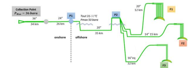
Fig 4. Injection Network Schematic with key nodes (P1, P2)
