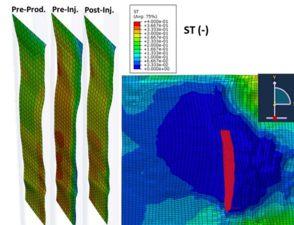
Fig 3. Fault Stability study outcome: Slip Tendency (left), Fault map (right)
