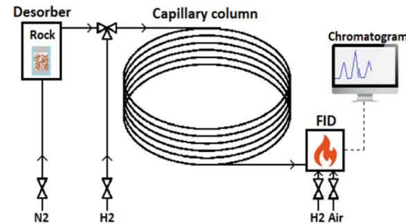
Fig. 1: TE-GC instrumental scheme
